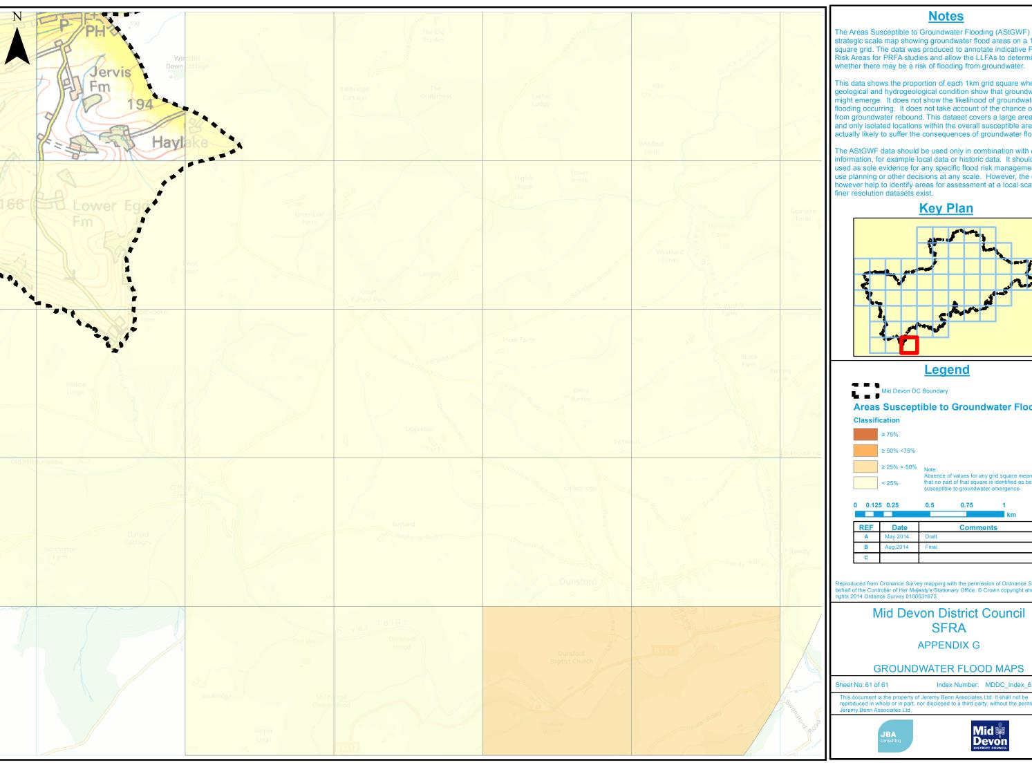
The Areas Susceptible to Groundwater Flooding (AStGWF) is a strategic scale map showing groundwater flood areas on a 1km square grid. The data was produced to annotate indicative Flood Risk Areas for PRFA studies and allow the LLFAs to determine whether there may be a risk of flooding from groundwater.
