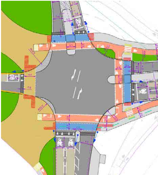
↑ Example of a signalised crossroads junction which delivers pedestrian and cycle crossings
